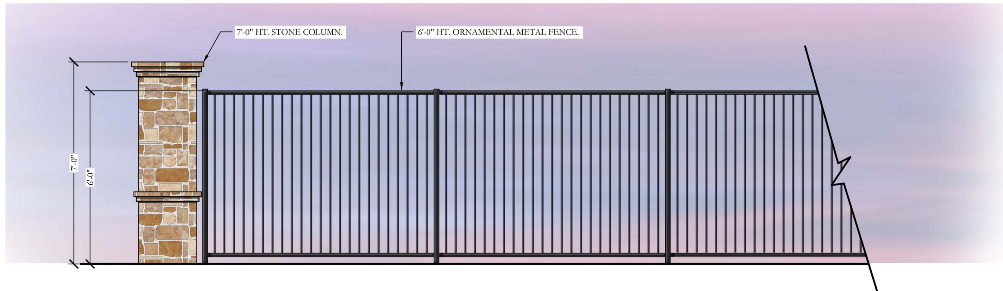
COLUMN WITH 6'-0" HT. ORNAMENTAL METAL FENCE ELEVATION
