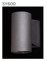
Syrios light module is designed with a tilting mechanism allowing forward and back light adjustability. The ±30° directional module allows to aim the light beam in the desired direction, without disturbing the luminaire mounting. The module can be secured using the built in locking mechanism.
